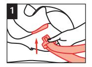
Thread both vehicle lap and shoulder belts through the slot (as shown) and out other side. Buckle. Pull up on shoulder belt until all slack is out and lap belt is tight.
